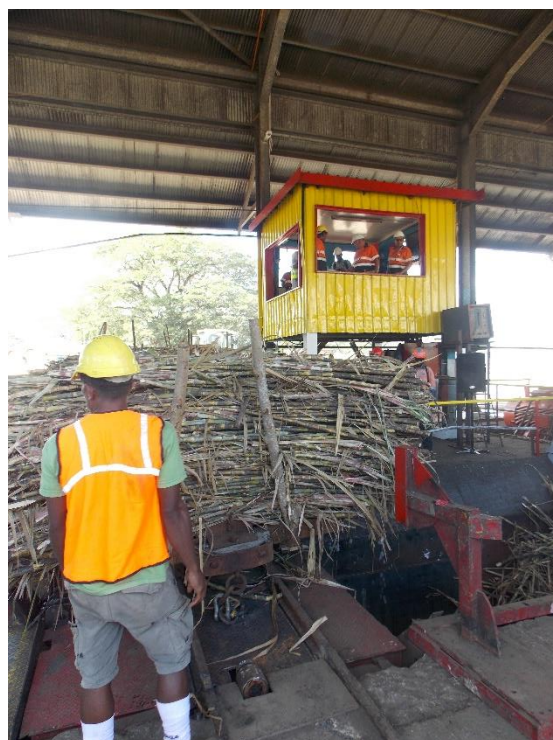
Above: Tipping of a cane rail truck at the Rarawai Mill opening this year
